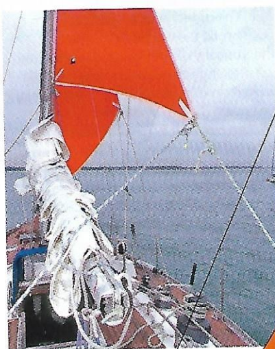
ABOVE Make sure the trysail is rigged before the heavy weather hits
