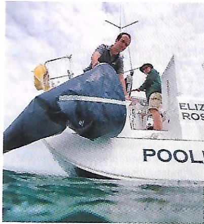
ABOVE Using a sea anchor or drogue will keep the boat's bow towards the waves, reducing the risk of a knockdown
