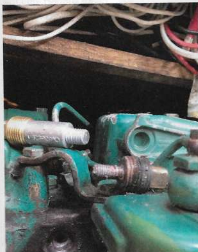
Engine anodes protect the internals of the cooling passages. They are a pencil-type that screws onto a short bolt that is itself screwed into the engine block. Some heat exchangers have similar anodes
