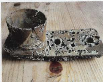
If the passive film on the surface of stainless steel is damaged the result can be pitting, caused by a galvanic reaction between the passive surface film and the active substrate
