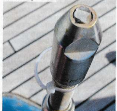
The top of the bottle screw head, where Garuda's rig failed
