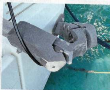
8. Borg Manduca on his new Dufour; (right) the damaged bracket from the Hydrovane
