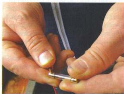
Using a multimeter to check a fuse is actually working – sometimes it's difficult to tell just by looking
