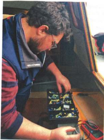
Looking for the correct size of fuse
