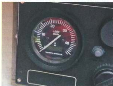
The engine was still running properly but the rev counter was at zero
