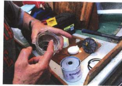
LEFT This is the primary filter unit with filter removed. Don't forget the O-ring! RIGHT Top tip: use Vaseline to keep seals in place during reassembly
