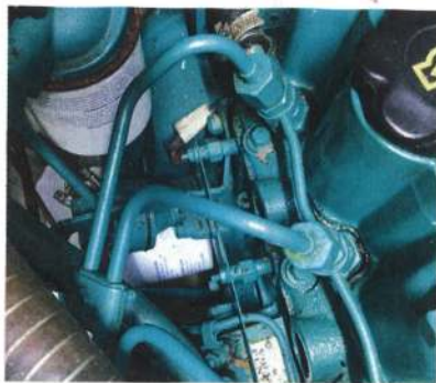
Oil filler cap (top right) secondary filter (top left) oil filter (bottom)
