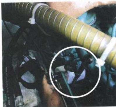
Stu uses a strap wrench to free the secondary filter
