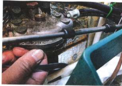
LEFT This is the primary filter unit with filter removed. Don't forget the O-ring! RIGHT Top tip: use Vaseline to keep seals in place during reassembly
