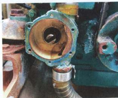
The impeller chamber is distorted to facilitate suction with the impeller vanes
