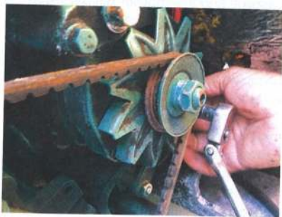
Stu loosens the alternator bracket adjustment bolts to change the drive belt
