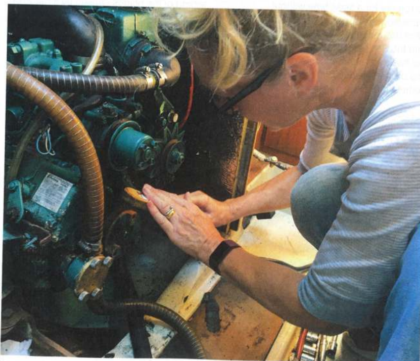
Laura removes rust from a pulley wheel with a wire brush
