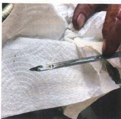
Checking the oil level on the dipstick
