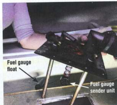
Hatch cover removed, you can now see the feed pipes and fuel gauge
