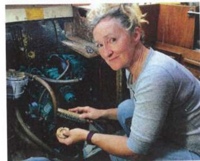
Laura cleans the Speedseal impeller cover with a wire brush
