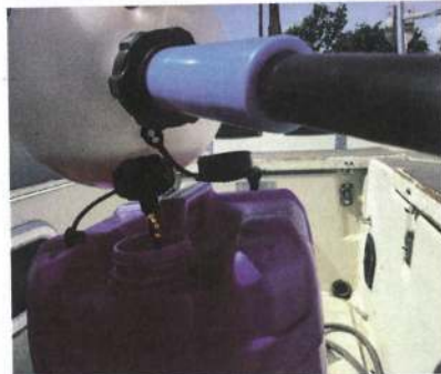
The pumped fuel is returned to a container and will go back in the tank
