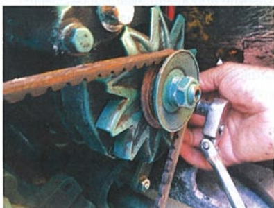
Stu loosens the alternator bracket adjustment bolts to change the drive belt
