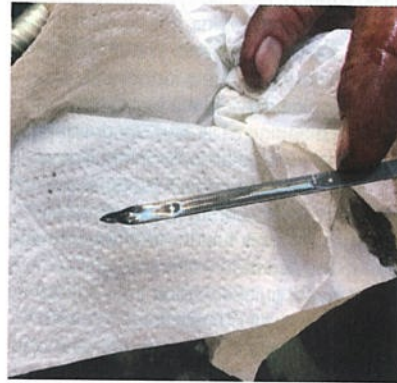
Checking the oil level on the dipstick
