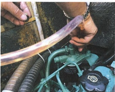
Clean fuel drawn into the secondary filter using the oil change suction pump. Note bleed plug in Stu's left hand
