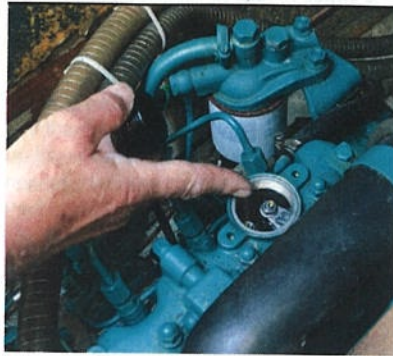
Oil filler cap removed from the rocker cover, ready for an oil change
