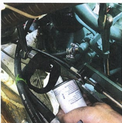
The secondary filter is removed
