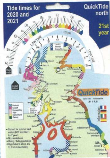
Figure 1: The QuickTide code for the day set at G0 for the worked example
