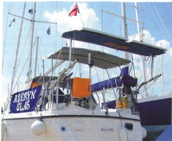
ABOVE Aderyn Glas is fitted with two monocrystalline solar panels which are rated at 100W apiece – they take the same space previously occupied by amorphous panels which could only muster 75W between them
