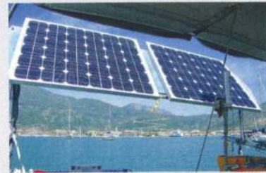
The tilting mount on Aderyn Glas allows us to track the sun's elevation
