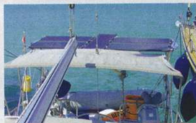
Stern mount keeps solar panels well away from stray shadows
