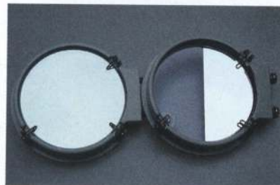
ABOVE The two main types of sextant mirror – either whole screen (left) or split screen (right) – display the view in different ways, and each has their advantages and disadvantages
