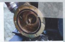
have paper gaskets) and while you're there, check the drive shaft seal at the back of the housing – a leak can seriously damage an engine.
