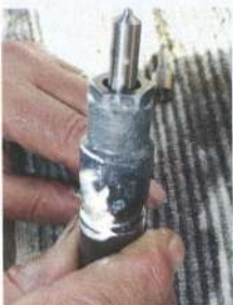
Injector body smeared in lithium white grease
