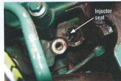
The clean injector seat can just be seen
