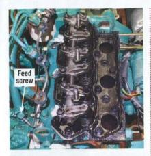
Next I removed the valve cover, which is retained by three dome nuts. I'd previously removed the injectors and protected the injector ports from contamination, and the new very expensive shiny fuel leak-off pipe can be seen on the left. This was removed and the feed screw placed back into the injection pump with both washers to prevent loss and contamination.
