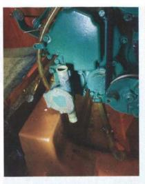
The raw water pump does not strictly need to be disconnected but it does improve access and as I had a full gasket kit, I took the opportunity to dismantle and replace all gaskets and seals, as well as change the impeller. The stop-cock for the raw water cooling which is built into the saildrive must be closed before disconnecting these pipes.
