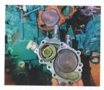
With all the bolts removed from the water pump, I was able to tease it off the engine, but there was still the backing plate to think of. It's tempting to use screwdrivers to prise it off but that method can damage the mating surfaces. It's best to tap it gently all round with a dead-blow hammer.
