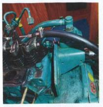
At the rear of the engine the bracket that holds the fuel filter spans the block and head so also needs to be detached. In hindsight I should have removed this before I tackled the exhaust elbow as it would have allowed easier access to the bottom inboard bolt which, can be tricky to get to. This does not need to be completely removed, just unbolted to allow the head to be removed.
