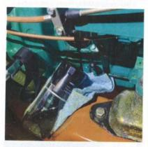
Draining the oil is not necessary in order to pull the cylinder head, but I was planning on doing a full service on the engine at the same time, so I removed the oil filter and pumped out the oil via the dipstick using a vacuum pump.
