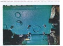
The heat exchanger is held on with four bolts and two studs at the rear. The studs are also used to mount the electrical box. I used two of the nuts locked against each other to later remove the studs from the cylinder head.
