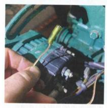
Sticking with the electrical theme, next to get disconnected were the water temperature sender, oil pressure sender and glow plugs.
