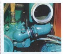
There are two pipes connected to the heat exchanger, one underneath and one at the front, both connecting it to the water pump. These were showing signs of cracking, so I purchased a replacement kit. I could now see that the front one would be very difficult to replace without removing the heat exchanger, so it made sense to get it done immediately.
