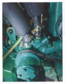
With all fluids out of the engine, disassembly can commence starting with the hot water hoses which typically go to the calorifier. The reason these pipes have insulation on them is that we also have a water-based heating system and all the piping is insulated to improve efficiency.
