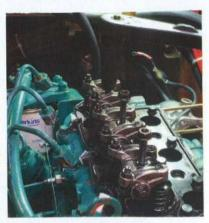
The rocker arm assembly needs to come off as it covers a number of the cylinder head bolts. An extra deep socket makes this process easier. While a spanner could be used for disassembly, a torque wrench is required when re-fitting, so a socket really is required. With rocker arm off the push rods simply lift out of the block. Store them carefully so they can go back in the same order they came out.
