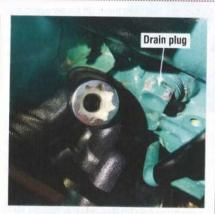
The cooling system will need to be drained, however. A good trick with this engine, which has a square drain plug, is to get a 17mm 8-point socket that fits the nut perfectly, then carefully drain and collect the fluid for correct disposal.
