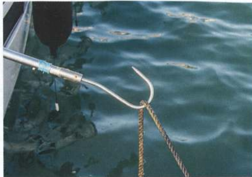
The blunt gaff on the end of a boat hook we prefer for routinely pulling the line forward
