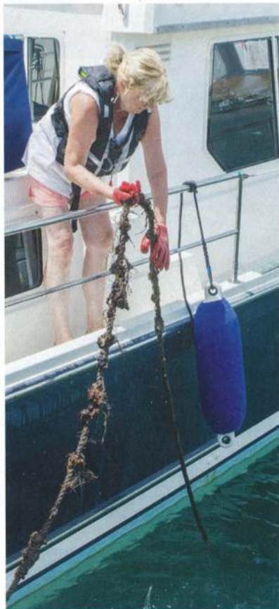
Gloves are essential to protect hands against marine growth on the lazy line
