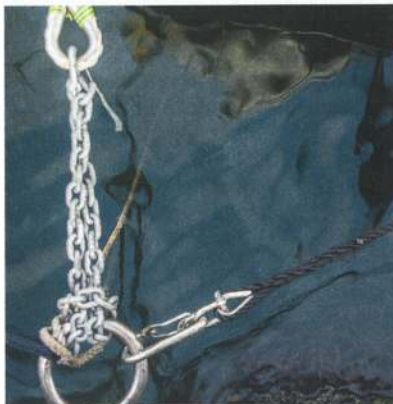
Hooks may be useful both for ease of attachment and to prevent chafing
