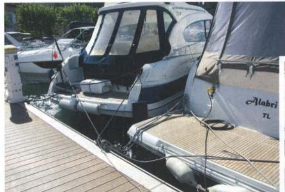
Here spring lines are stopping the boat from moving around too much. Notice that the further boat has swung around while the nearer boat hasn't. Part of the reason for that is that bow and stern lines may be tighter on the nearer boat limiting its movement. Fendering between boats remains important even when moored up
