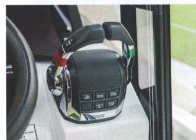
Colour coding also used to identify throttles on a twin engine boat
