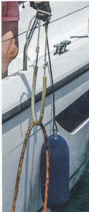
Using a rope loop (covered in plastic tubing) to pull the lazy line forward. This enables you to use the rope loop to tie off the lazy line temporarily. Note there is only one hand loop spliced into the loop so the hand can't get trapped
