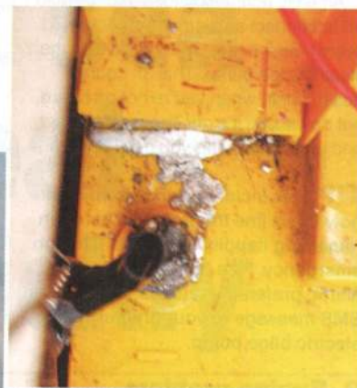
ABOVE Most of this battery terminal vanished into a puddle of molten metal due to a crack in the clamp
