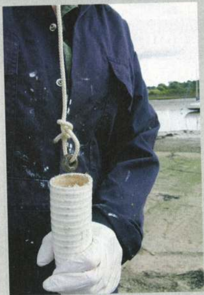
Drop a line through the pipe and use it to draw a bottle brush back and forth
