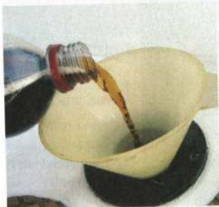
Descaler (in this case vinegar) is poured into the system via the holding tank out 'filler' on deck
