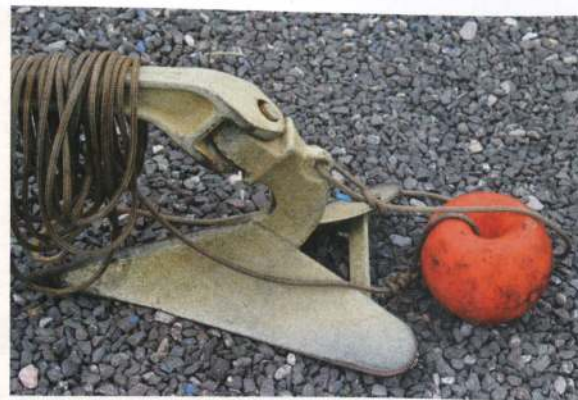
Tripping line and buoy attached to the tripping eye of the anchor
