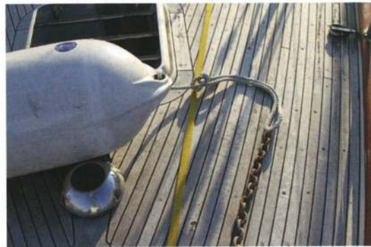
ABOVE LEFT A lashing preventing the cable jumping out. A split pin between the two cheeks is also an option.
