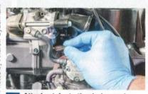
Attach a tube to the drain nozzle, putting the other end in a container.
