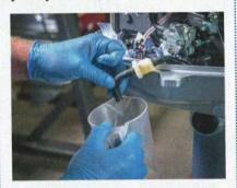
Feed the line into a suitable container and open the fuel line.
