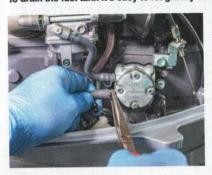
With fuel tap off, detach the clip holding the fuel line to the fuel pump.
