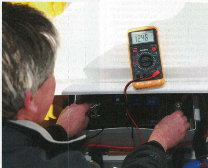
A voltmeter attached direct to the battery terminals gives the most accurate reading
