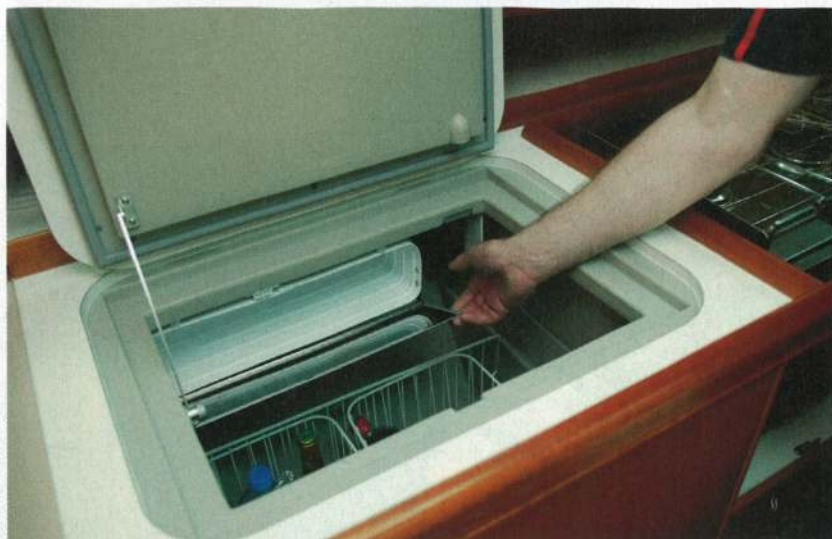
Simply improving fridge insulation can reduce power consumption on board
