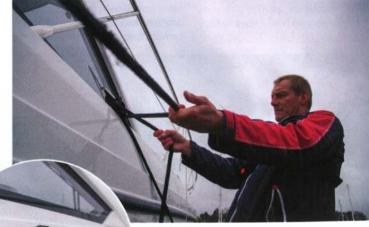
6 SWEATING IN The spring lines should be nice and taut, so sweat them in by leaning on the standing part and taking up the slack. The second spring should have the full 0880 to keep it secure. Locking turns aren't needed if done correctly.
