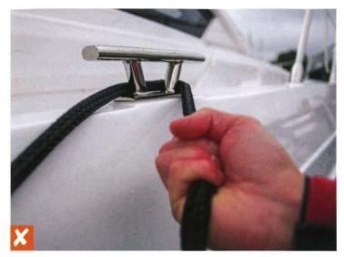
**1 INCORRECT LEAD** The way you lead the rope around the cleat is crucial to tying up a boat correctly. Here, the lead is the wrong way around the cleat and is described as 'closed'. The weight and wear are on the toe rail instead of the cleat, causing premature wear to the gelcoat and the rope. It also makes it difficult to tension the line by 'sweating' it in.
