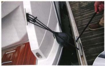
**3** BOAT TO SHORE When running a sternline from the boat to the shore, it has to go from the boat's stern cleat to a pontoon cleat located a little way aft of it. A bowline has to go forward. To ensure the lead is correct, always go to the furthest side of the cleat from the boat to keep it open and don't pull it too tight.
