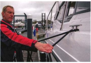
**5 SPRING LINES** Once the bow and sternlines are secure, they can now be returned up to the mid cleat to become stern and bow springs. As many boats only have a single centre cleat, you may have to use a simpler 080 in order to leave enough space for the second spring to be made off here too.
