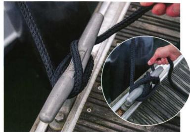
TYING OFF To make off a line to a cleat, take a turn around the base (0), followed by two crossing turns around each horn (88), then a second turn around the base (0) to leave an '0880' shape. This grips the cleat well and allows an easily controlled release. It also leaves the tail pointing in the right direction to become a spring line.
