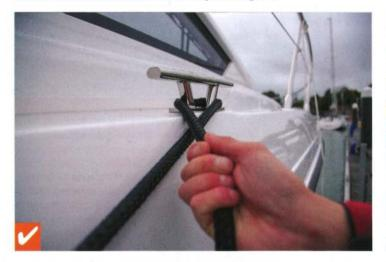
**2 CORRECT LEAD** Now the wear and weight of the boat is on the cleat not the gelcoat. You or your crew can now assist with tensioning the line by keeping the line taut with your right hand while pulling on the standing part of the line and sweating in the slack.
