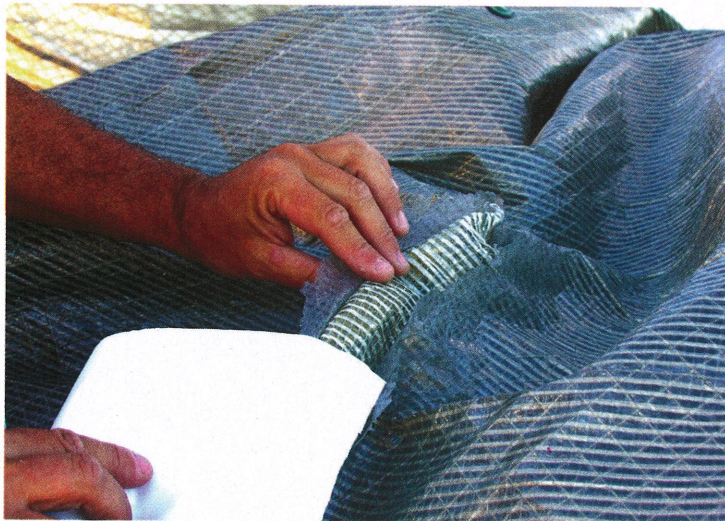
A roll of sticky-backed Dacron is invaluable for emergency sail repairs large and small
