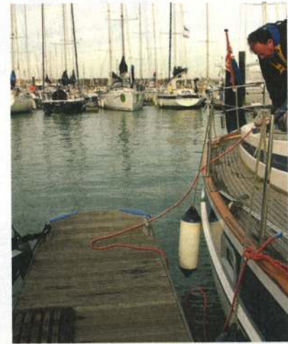
4 I take the slack out of the line, being careful to keep the cleat lassoed
