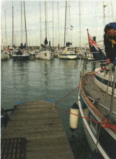
5 With two turns round the winch click into ahead and drive against the bridle
