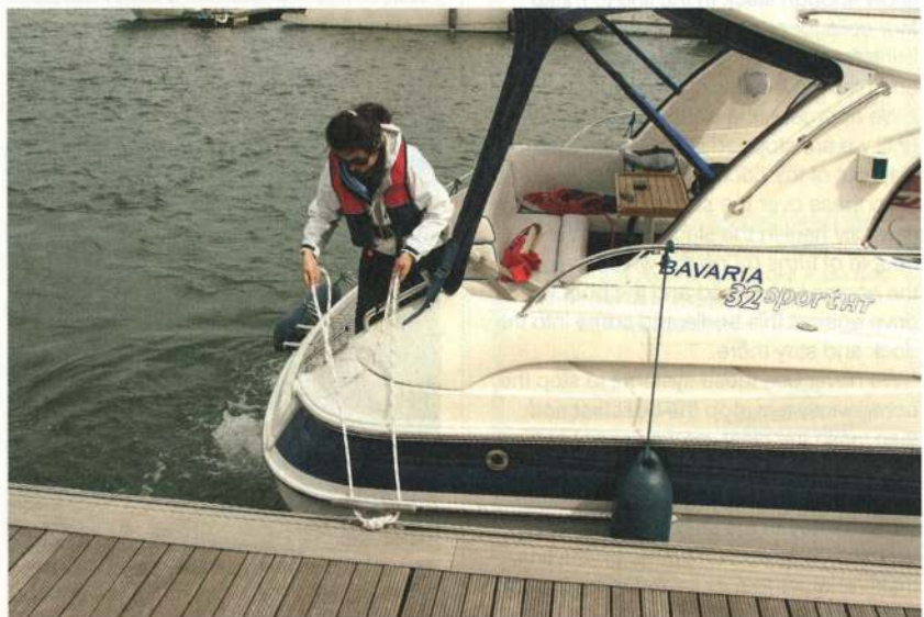
The loop is simply dropped over the mooring cleat...
