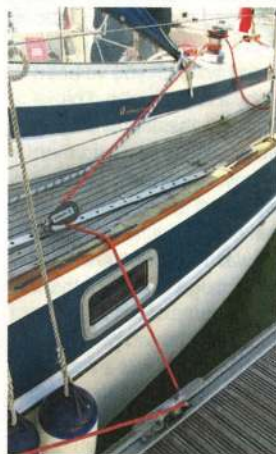
Bridle returns to boat further forward via a block on the genoa sheet lead, to allow for a shorter finger
