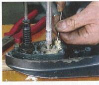
Next remove the impeller dowel pln from the drive shaft.
