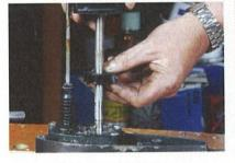
The lower unit can now be set up on the bench ready for disassembly of the water pump. Remove the four bolts along with their support plates and slide the pump housing and impelier up the drive shaft.
