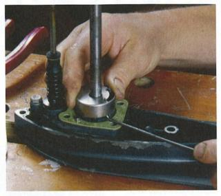
Smear the Inside surface of the Insert with waterproof grease and gently lower it onto the impelier, slowly turning It anti-clockwise to deflect the impeller blades and allowing it to silde into place. Any errant impeller blades can be gently eased home using a screwdriver.
