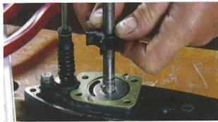
The new face-plate is fitted onto the water pump base, Installed dry without sealant. This is followed by the gasket lightly smeared with gasket sealant. The new dowel pin is then fitted and the new Impeller slid down the shaft onto the pin.
