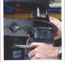
Once the lower unit starts moving it can be drawn off the leg as the water feed tube, shift rod and drive shaft become disconnected within the leg.
