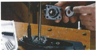
The pump body includes a metal insert but it's easiest to slip this over the impeller before installing the pump body.
