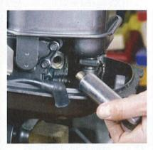
Pull off the plug lead and remove the spark plug using a proper spark plug socket with rubber insert to prevent the ceramic part of the plug being broken. If you don't have one use a standard deep socket, taking care not to apply any sideways pressure to the ceramic part of the plug with the top of the socket.
