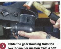
3 Silde the gear housing from the leg. Some persuasion from a soft faced hammer will almost certainly be necessary to break the corrosion seal between the two parts, but light tapping should be all that's required and will avoid distorting the cavitation plate.
