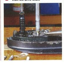
Fine wire wool gives a good clean surface finish to the water passages although there is nothing to be done about pitting of the surfaces. The drive shaft can also be cleaned of corrosion and salts using fine wire wool. Now you can begin reassembly.
