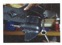
Remove the two bolts and washers that secure the gearbox housing to the leg. Note the ring anode just ahead of the rearmost bolt. While the lower unit is detached, remove this and either clean the scale off or replace it with a new anode.
