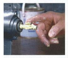
Smear the propeller shaft generously with waterproof grease prior to reassembly. The propeller nut should be tightened sufficiently to hold the propeller firmly against the shear pin before the locking pin is refitted. Other makes of motor may differ in this respect.
