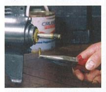
Remove the shear pin and check it closely for cracks or bending. If it shows signs of serious wear replace it with a new one of the correct size and type. Don't substitute it for a high tensile bolt with the idea of preventing it breaking – it's there to protect the prop from excess damage in the event of it striking hard bottom or floating debris.
