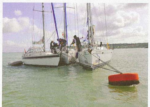
To leave the raft, again downtide, the middle boat slips springs, then stern and bow lines, then slips its mooring line and glides out gently, minding rigs. The two remaining boats glide together but don't forget to fender the bow
