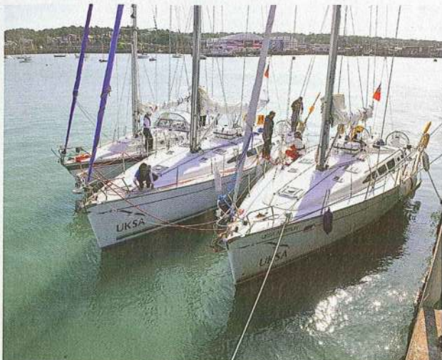
Without another line long enough the outside boat is using its shore line as a new bow line, run around the bow of the middle boat, which is the one departing, to the inside boat
