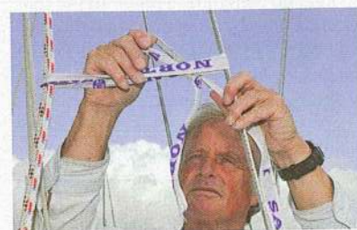
Make sure your halyards are frapped away from the mast so they don't spend the night clanging against it
