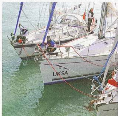
The middle boat has dropped its stern lines and is now slipping bowlines in readiness for leaving downtide, which means astern in this instance. Middle and outside boats have their engines running — just in case
