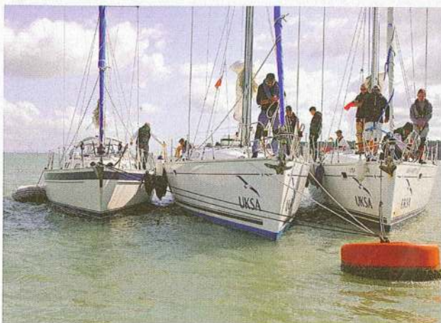
Three approaches to mooring to a buoy: the middle boat has rigged a bridle, the boat on the left has rigged a round turn with a bowline long enough to be untied from deck. The boat on the right will need to be creative slipping its mooring
