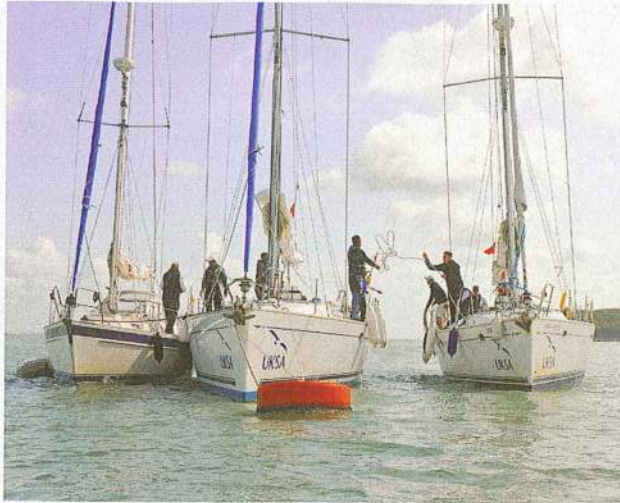
Having asked to come alongside, bow and stern lines are passed to the central boat, then springs are rigged, making sure the spreaders won't clash, starting things off badly
