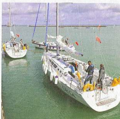
The middle boat has slipped and run astern out of the raft. With the new stern line now properly rigged, the outside boat begins to haul on both bow and stern lines to get back alongside the inside boat
