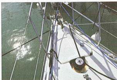
If all the cleats are full, there will be other strong points on deck that can be used. A tugboat hitch on a winch or windlass will serve well if needs be
