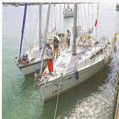
Bow and stern lines are secured, followed by springs, then new bow and stern shorelines will be rigged to finish the job and attach the remaining yachts in the smaller raft
