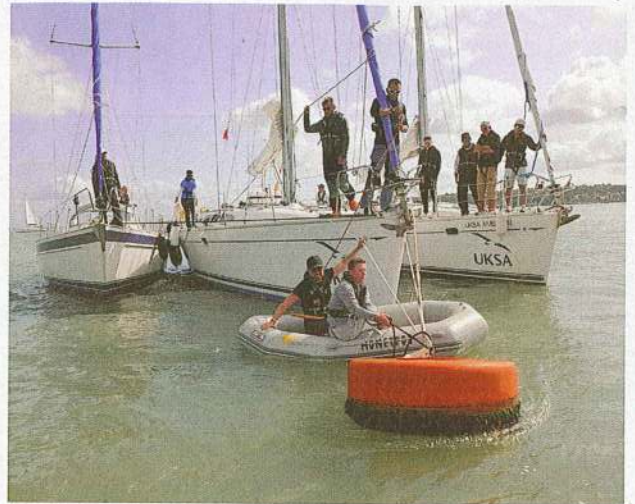
All boats need to run their own mooring lines to the buoy, which is most likely to involve a tender
