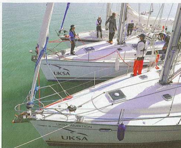
The outside boat runs a new stern line around the bow of the middle boat and back to the stern of the inside boat. The line will be rigged when the middle boat has begun to leave
