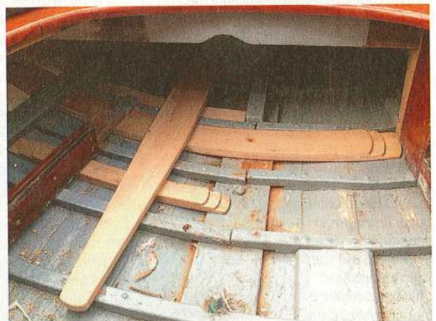
A laminated oak backbone spread the weight and torque of the motor
