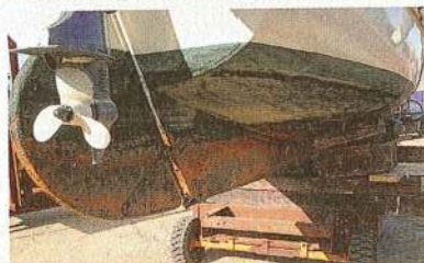
No aperture in the rudder for a prop
