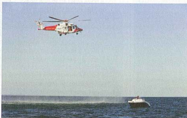
1 The boat has stopped and is lying beam-on to the wind as the helicopter hovers downwind, keeping the downdraught clear.
