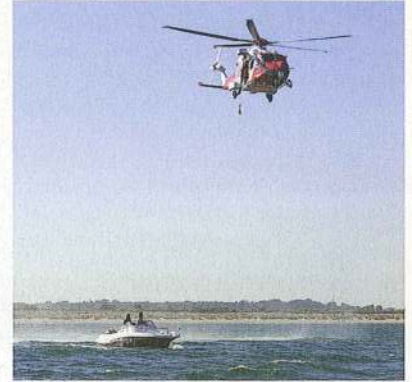
3 ...before beginning to lower the weighted winch line.
