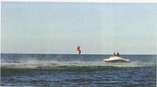
3 As the helicopter brings the winchman in closer, the downdraught comes ahead of the boat and the bow points further downwind.
