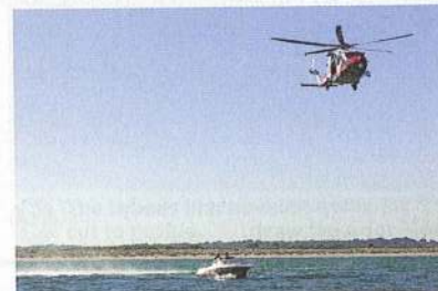
Approaching from the port side allows the helicopter to maintain visual contact
