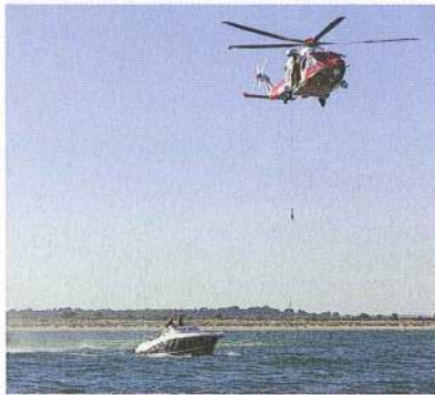
4 An earthing line is on the end of the winch line and should be allowed to make contact with the boat or the water before being touched by the crew on the boat.
