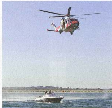
5 Here the line ('winchman') is close to the boat, but the aim is to lower it (him) into the cockpit rather than on to the bow.
