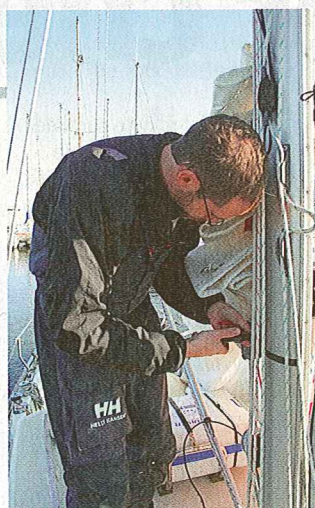
Check the gooseneck for excessive movement
