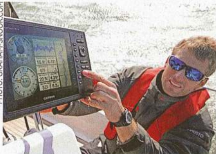
Theo takes a plotter screengrab to record the data onto an SD card
