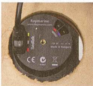
Raymarine's rectangular Seataalk ® connectors are easily spotted
