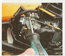
The throttle cable is connected by a locking screw on top of the carburettor. Because adjustments may be required on refit, make relevant notes (eg cable tail lengths) or take pictures of anything you remove to make refitting of components a little easier.
