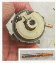
The main jet when unscrewed has a nozzle tube above it which feeds fuel directly into the carburettor chamber. However, because the engine would now run well in gear and under load, but still not tick over properly, I knew that the problem was with the idle circuit in the carburettor.
