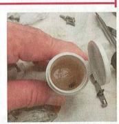
After freeing the hole I then left the jet soaking for about an hour in carburettor cleaner. It was much more clean when it came out, and I put the carburettor back together and refitted it to the engine – which now idles perfectly. The carburettor cleaner cost £6.99 and the screwdriver £6.55.
