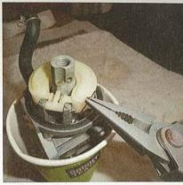
The main jet looked clear, but a paper cup proved an ideal soft, flexible holder while I gave it further sprays to soak it and then used a fine needle to carefully clean any of the larger holes.
