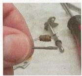
A single strand from a bike gear cable proved the ideal diameter to initially clean the hole.
