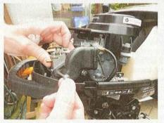
By carefully withdrawing the long bolts the carburettor could then be lifted clear, but take care to keep it upright to avoid any residual fuel spillage
