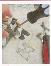
I did not have a suitable size screwdriver to unscrew the jet, so I ordered one online from RS Components. It was a Wera 3335 screwdriver, and the blade was 4mm wide by 0.8mm thick and 100mm long.
