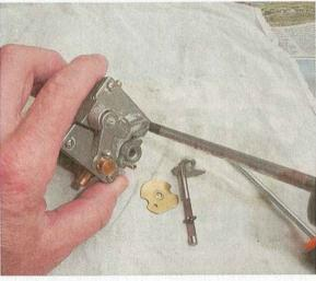
The top plate can then be unscrewed. In this case it could be slid out from under the throttle mechanism, which may have to be removed on other motors. The thing to remember is not to remove anything you don't have to.
