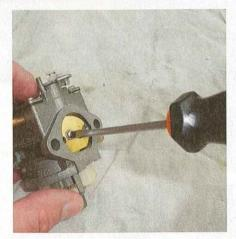
The pilot jet for the idle circuit is located under the top plate housing of this carburettor. To remove the plate I first needed to take out the choke. The brass disc which incorporates the choke flap can be unscrewed.
