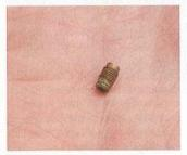
The pilot jet is very small, but when I removed it I could see that it was clogged with residue.
