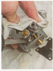
Now I had access to the pilot jet housing. The jet itself sits under a chrome screw which could be removed with a standard screwdriver.
