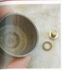
The bowl, when removed, can be thoroughly cleaned of any debris or residue. Note the locking nut has a washer, so carefully retain this or replace if necessary.
