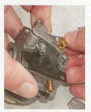
Underneath the top plate was a rubber membrane which could also then be taken off. When inspected, this was in good condition so it could go straight back on again afterwards.
