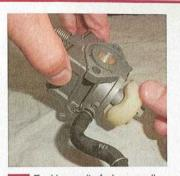
Fuel is gravity-fed on small outboards. The carburettor bowl has a plastic float suspended in the fuel chamber, and when the fuel drops below a certain level it sinks and opens a valve to allow more fuel to enter the bowl. Check that the float moves freely, but be careful because it has delicate springs.
