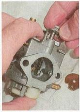
The mounting spindle for the choke flap can then be withdrawn. Do this with care, because it has a small O-ring at the top through which the choke shaft rotates open and shut.
