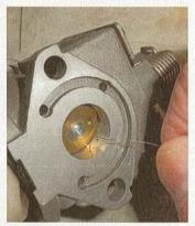
Shown here is the throttle flap; fine fuse wire was used to make sure the small holes were clear. At this point I refitted the carburettor and the engine performance improved, and now it would idle for a short time but then cut out.
