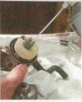
I had tried to use carburettor cleaner with the engine running, without success. However, with the carburettor removed I could spray it directly through the main jet and other accessible ports.
