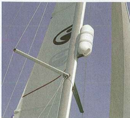
Passive radar reflectors can do only so much. Consider an active radar target enhancer
