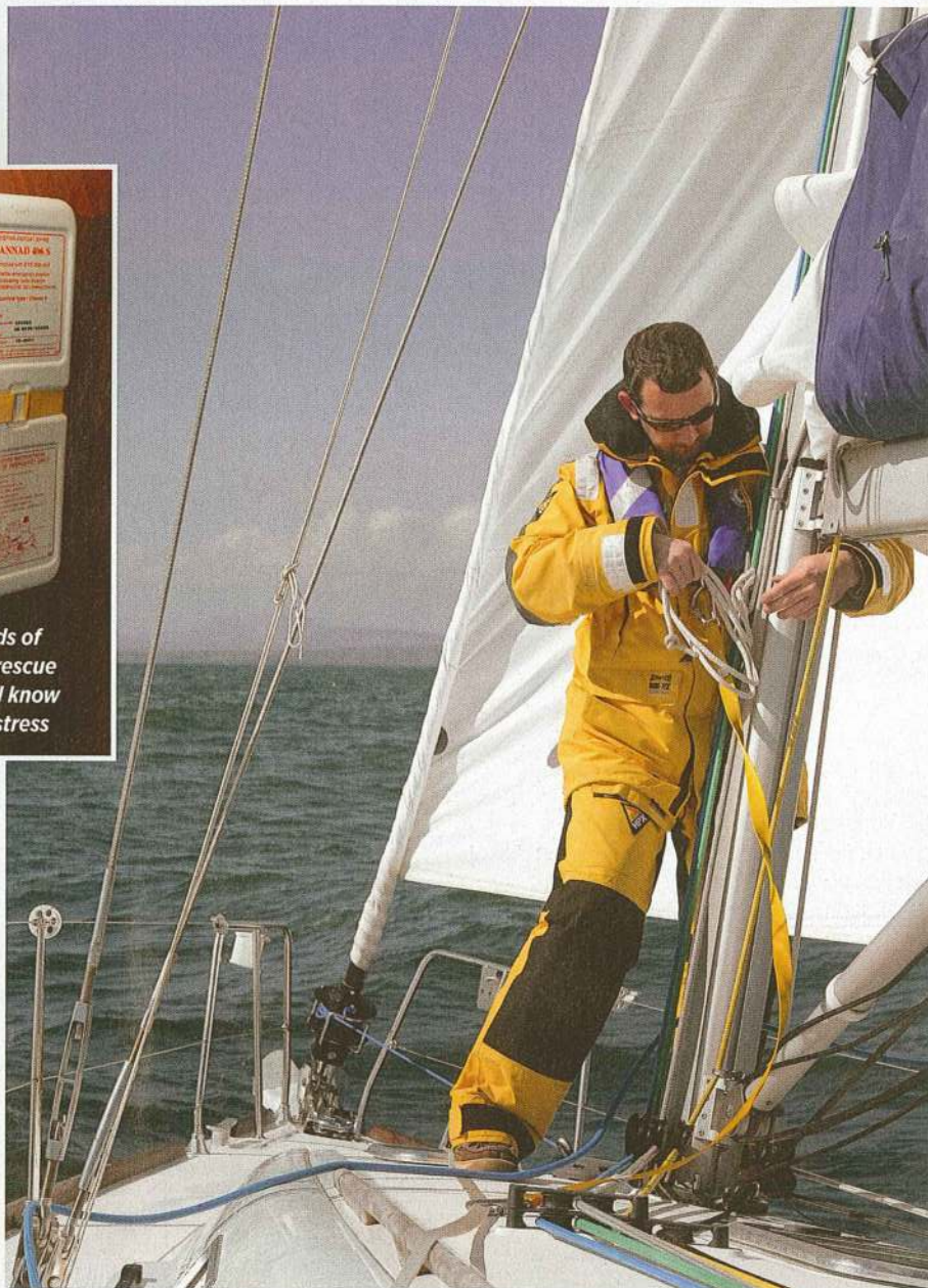
Clipped on while working at the mast, but the jackstays aren't tight and the tether is too long
