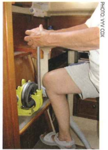
YM's Vyv Cox has a high volume manual bilge pump that bolts onto the companionway steps
