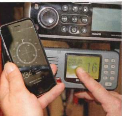
Check that the DSC VHF is hooked up to the GPS, and that it's reading out a sensible position
