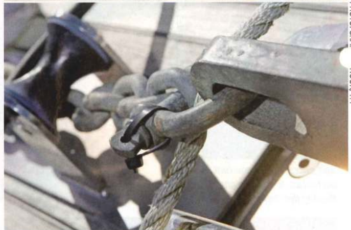
TOP: Flush pins on this Kong swivel - no need for any seizing here ABOVE: A cable tie should let you see the week out
