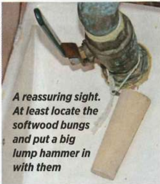
Locate all your seacocks and check that each of them is sturdy and turns smoothly
