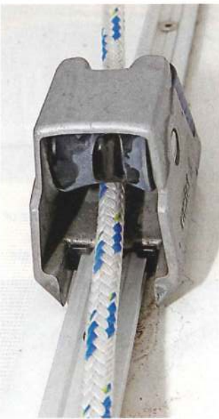
The chafe and friction from worn or cracked sheaves on turning blocks or sheet cars can make a misery of any charter
