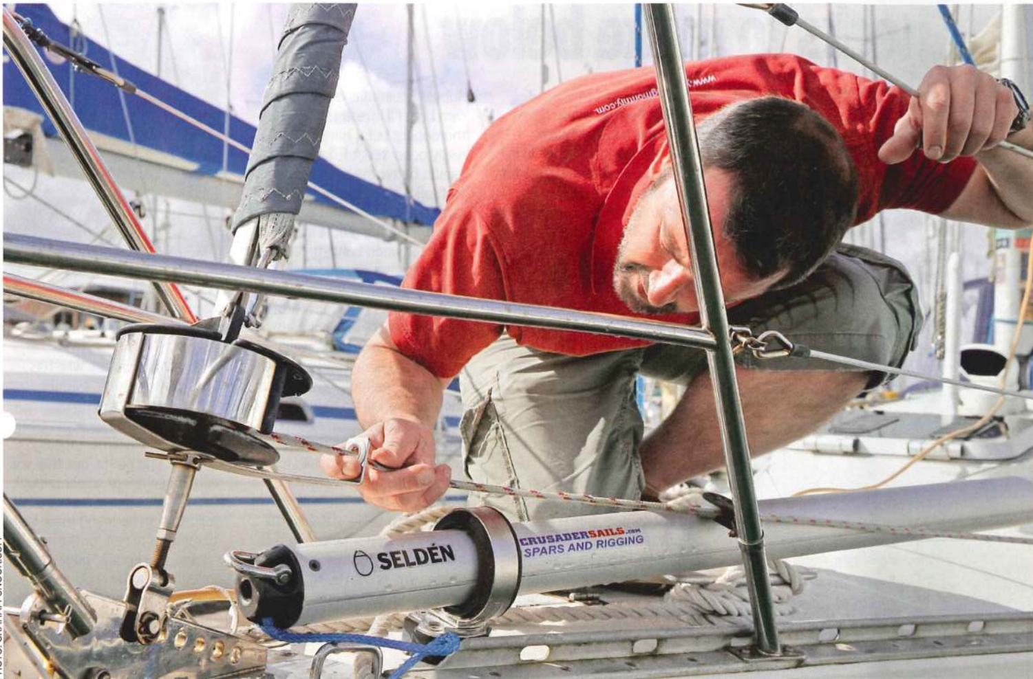
Check the furling gear has a decent lead, a healthy furling line and that the drum runs freely
