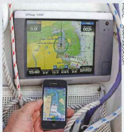
Check the plotter works and is hooked up to the GPS. Bring your own back-up device to pre-empt any problem with it
