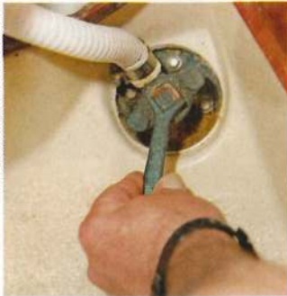
Locate all your seacocks and check that each of them is sturdy and turns smoothly
