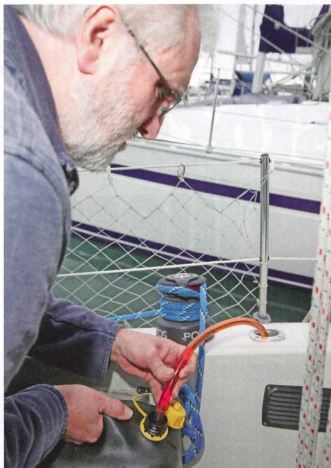
Top up with fresh diesel to avoid condensation forming in the fuel tank
