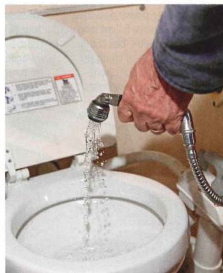
Pump the heads through with fresh water
