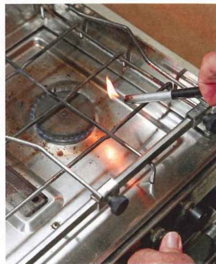
Burn off any gas and disconnect the bottle
