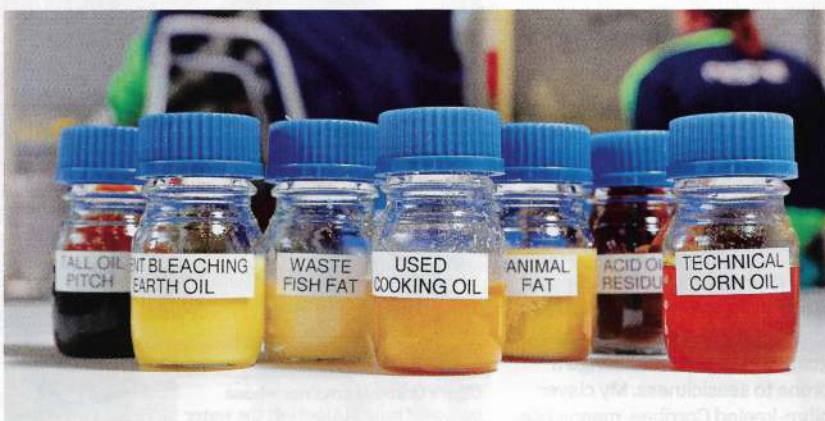
ABOVE HVO can be made from a number of different feedstocks including used cooking oil and animal fat waste
