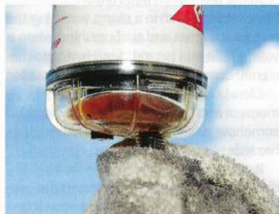
ABOVE Bio diesel is more hygroscopic than traditional fuels which means it holds water, increasing the risk of diesel bug
