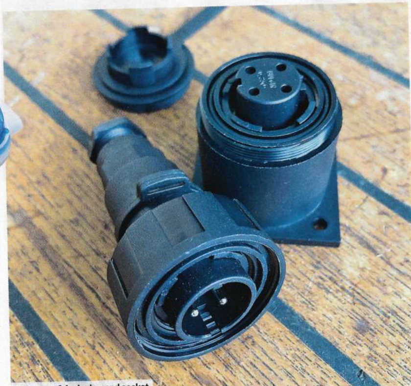
Waterproof deck plug and socket
