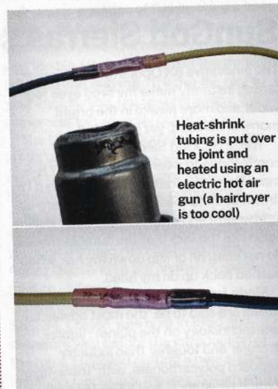
The tube shrinks to tightly grip wire and joint
