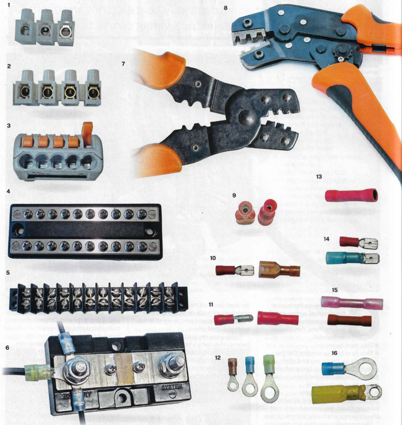
ABOVE 1. These connector blocks have a clamping leaf which is pushed down by the screw to hold the wire 2. Without a clamping leaf, as here, there is a risk of breaking the strands of wire 3. Alternatively there are Wago blocks which don't use screws, but have a spring contact 4. Marine grade 'bus bar' connector 5. Multiway connector block 6. Use crimp eye terminals – no more than four to a single screw or post 7. Non-ratchet crimping tool 8. The better ratchet crimping tool 9. The much better double crimp (left) and the cheaper single crimp (right) 10. Spade connectors – male and female to fit into each other 11. Bullet connectors – male and female to fit into each other 12. Ring terminals 13. Butt crimps 14-16 All these connectors are available with a heatshrink sleeve (second in each pair), which helps waterproof the connector, or not (first in each pair)
