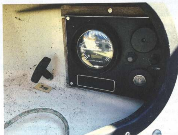
LEFT The engine is started with a cranking battery. Very high loads are delivered for a few seconds and this is restored by the alternator once the engine is running. If the revs drop (as they later did!) this could be an indication the alternator isn't working
