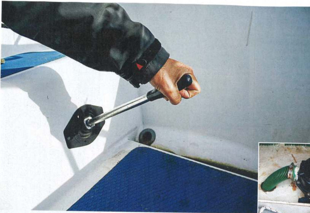
LEFT Manual bilge pumps should work with all cockpit seats in place and hatches shut
