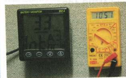
The 25A test set-up, with battery, discharge meter, data logger, ammeter and voltmeter
