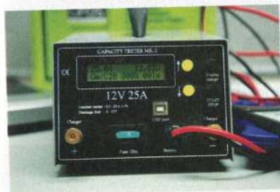
The MK discharge tester takes a constant 25A, and shows the capacity on a screen
