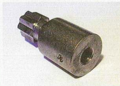
The Cranker is a converter that replaces the chuck on a right-angle drill
