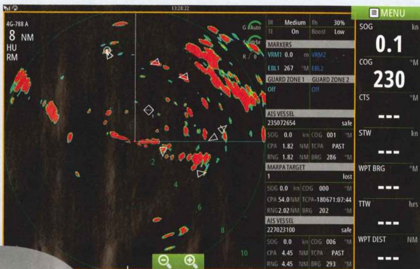
ABOVE: Tracking multiple MARPA and AIS targets on one screen
