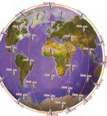
Above: Iridium's network of 66 satellites buzzing around Earth give global satcom coverage
