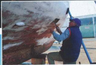
ABOVE In Portugal Wendy May was lifted for some work in a local boatyard: here the shipwright is cutting out and fixing a bit of rot TOP Looking smart with a new coat of paint
