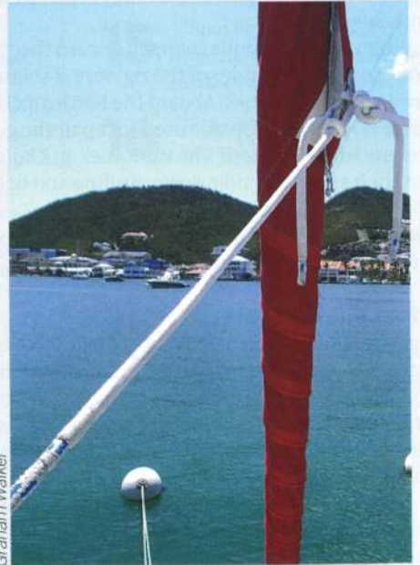
Dyneema chafe sleeves installed over the first 2m of Barracuda of Islay's genoa sheets help to reduce sheet wear when running downwind
