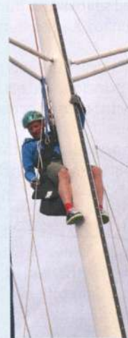
Left: the radome came adrift on Umoya of London during the first night of the ARC. Crewmember Jerry Norton went aloft to remove the sharp-edged remnants of the remaining fitting on the mast. Below: the damaged radome and broken parts of the shattered mast bracket
