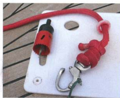
A plastic chopping board was called upon for a makeshift repair aboard the Beneteau Oceanis 55 Julia . Skipper Louie Neocleous said the spinnaker halyard exits the masthead and runs down the mast about 100mm to a metal fairlead. "Despite having a chafe sleeve... there was nothing to stop the metal snap shackle being hoisted too high up onto the metal fairlead. We knew we had to install some sort of stopper, so we improvised using a plastic chopping board."
