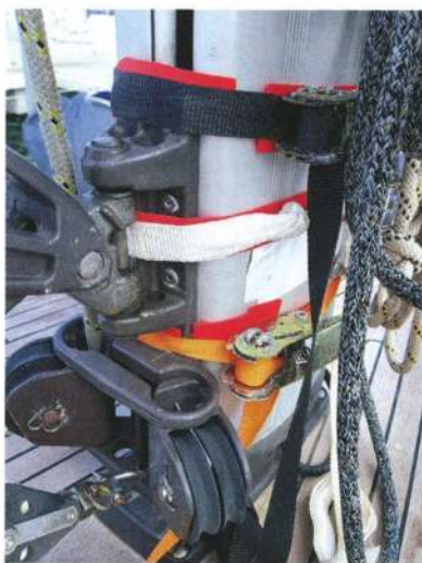
A spare mainsheet (top) was used for support and a red IKEA kitchen chopping board was cut into strips to stop ratchet strops chafing when pop rivets failed on Indian Summer's boom vang
