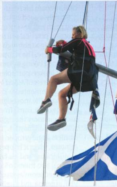
Aloft in a bosun's chair to install pipe lagging on the spreader ends aboard Barracuda of Islay – a move to combat chafing of the sails
