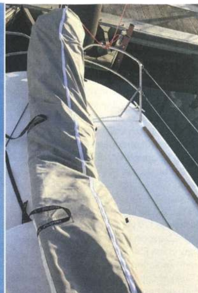
ABOVE Hank on jib with sail cover enabling it to be stowed on deck
