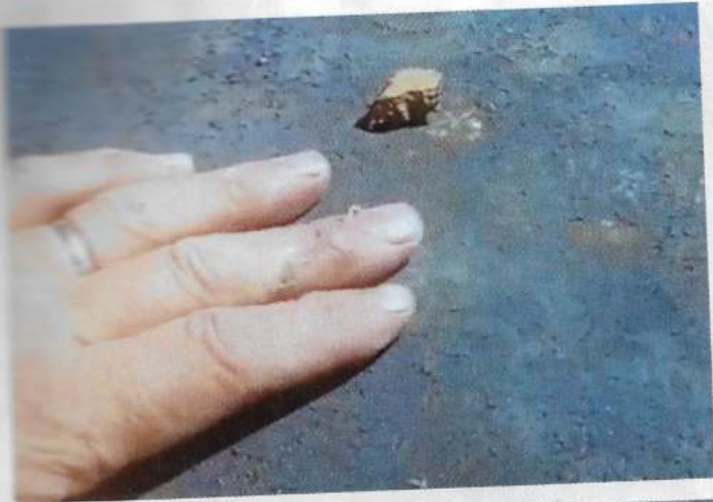
LEFT Water ingress to a balsa core deck. Not a good sign if you can flex it easily with your hand!
