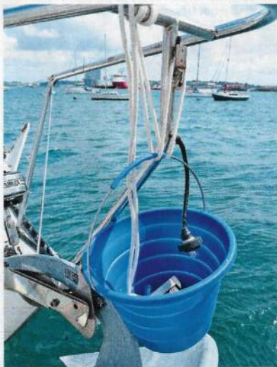
Be prepared for simple fixes such as corroded connections in navigation lights. The bucket will catch dropped components or tools
