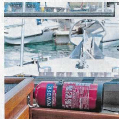
ABOVE Note that this fire extinguisher is located near an exit so if you can't put the fire out you're not trapped
