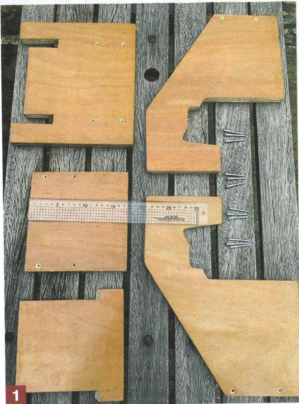
1 The components of the ply bracket laid out and ready to assemble
