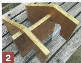
2 The hooks slot into the central base plate
