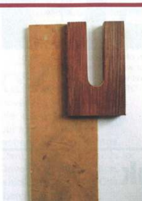
MDF fitting guide for position and perpendicularity
