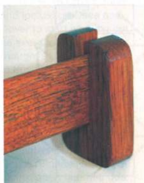
ABOVE and BELOW The pair of brackets glued to the bulkheads with Sikaflex
