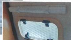
LEFT The finished blind in situ BELOW Velcro loop was used to secure the blind when closed
