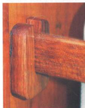
ABOVE and BELOW The pair of brackets glued to the bulkheads with Sikaflex
