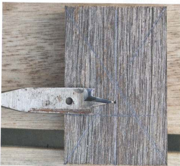
ABOVE Support bracket marked up for drilling
