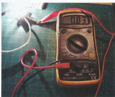
A 10W halogen bulb draws 0.83A
