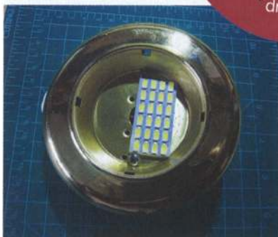
A single LED array fits easily inside the brass light housing
