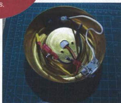
Back side of light housing. The LED driver is hidden inside black heat-shrink tube
