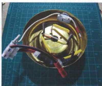
Rear view of a double array light. Note the two LED drivers in black heat shrink
