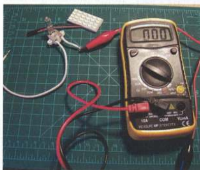
Checking power draw with a multimeter
