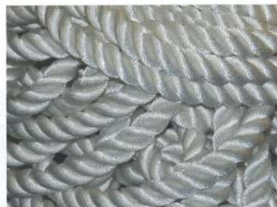
An example of a modern Nylon rope, hawser-laid
